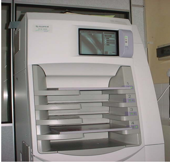
Fig. 5 A computed radiography (CR) reader. Shown here is a model with four input trays for simultaneous reading. Rigorous QC tests are necessary to produce optimum image quality. (Courtesy of Fujifilm)
