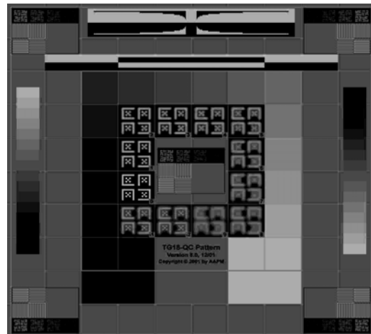
Fig. 4 The TG18-QC test pattern. The pattern contains: (1) 16 luminance patches at the corners of each of which are four low contrast targets for evaluating luminance and low-contrast response; (2) two continuous grayscale ramp bars for evaluating display bit-depth; (3) Cx and line- pair targets at the center and four corners and a scoring Cx reference for evaluating display resolution; (4) white-black bars for evaluating video artifacts; and (5) 5% and 95% embedded patches and low-contrast "QUALITY CONTROL" letters with variable contrast within different luminance backgrounds, for evaluating the grayscale rendition/ luminance response of the display device.
