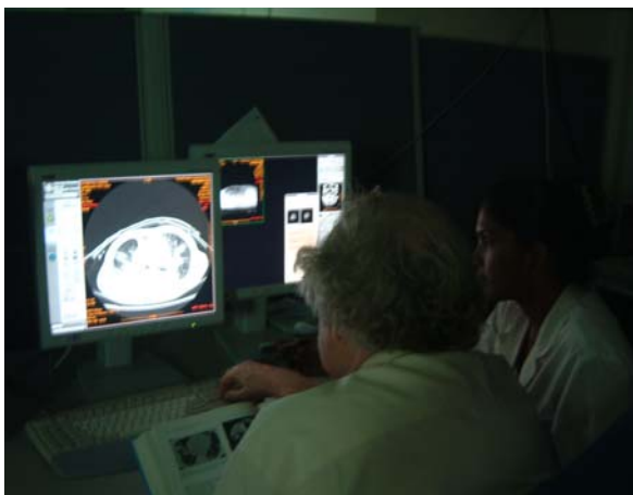
Fig. 2. A critical component for accurate diagnosis in a digital imaging department is the image display workstation where the radiologists observe the images to make a diagnosis. All clinical information passes through the display. Note the low ambient lighting condition.
