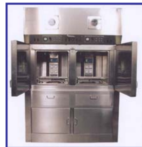
Hot Cell for automated production of radiopharmaceuticals
